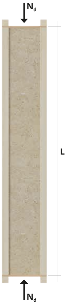
The dimensioning N_d capacity is calculated for load duration class medium and climate class 1. The table is based on the rules in SS-EN-1995-1-1, EKS11.
