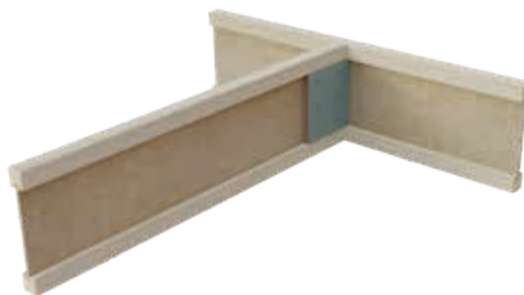
Connection with particle board reinforcement.
