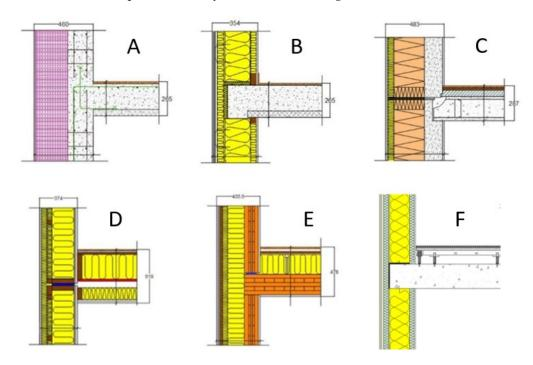
Figure 3 Detail of the exterior wall/slab connections in A) cast-in-place concrete with load-bearing outer wall, B) cast-in-place concrete and lightweight curtain wall, C) prefabricated concrete with load-bearing outer wall, D) volume elements of wood, E) CLT F) Pillar deck, concrete prefab and steel pillars / beams, light gauge curtain wall.
