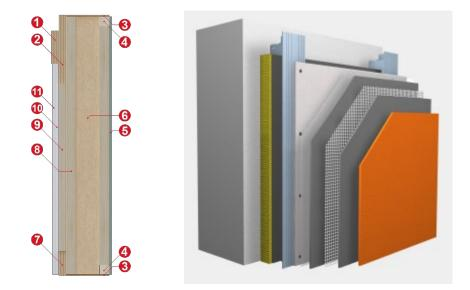
Figur 6 Exterior wall construction up to exterior panel ; 1) LVL 33 mm, 2# LVL 33 mm, 3) hardboard 6 mm, 4) blockings 45 x 45, between Masonite studs, 5) Fermacell 12,5 mm, 6) Insulation, 7) LVL 33 mm, 8) R200, c600 + 195 mm Termoträ, 9) 34×95 c600 + 45 mm Termoträ, 10) Fermacell fire panel 15 mm, 11) Fermacell 12.5 mm.
