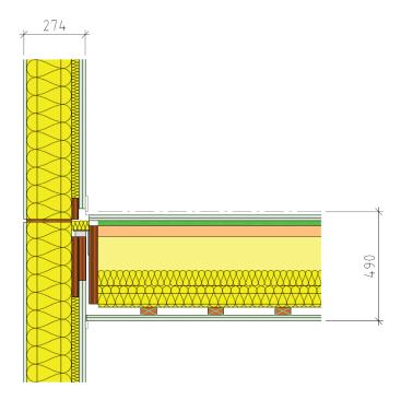
Figure 5 Overarching floor structure and outer wall. The outer gypsum fibre board is faced with an aluminium profile and an additional external plaster-bearing board which provides an aerated facade, see Figure 5 below.
